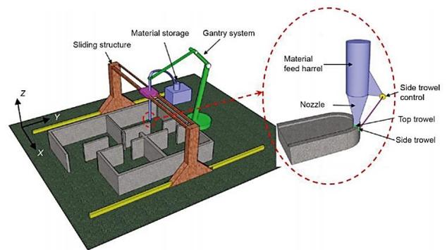
Fig. 5. Shows 3D printing during build construction MA GuoWei1, WANG Li & JU Yang" State-of-the-art of 3D printing technology of cementations material—An emerging technique for construction"2017-scince china- Technological Sciences
