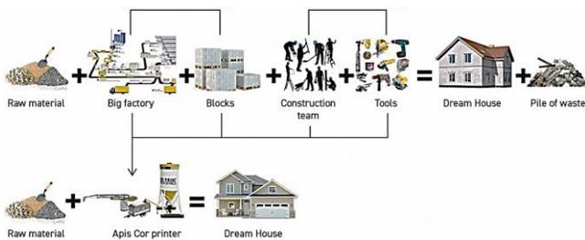
Fig. 3. The difference between traditional building and 3D printing [https://medium.com/@Nik\\_chen/what-is-construction-3d-printing](https://medium.com/@Nik_chen/what-is-construction-3d-printing) (date 29/1/2018 11:05pm)
